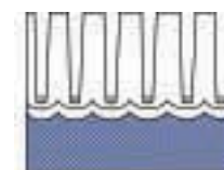
2 - Color added to bottom of coating pores.
