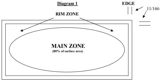
When inspecting a piece of glass you should be standing 10 feet from the surface of the glass and at a 90 degree angle perpendicular to the glass surface. (Inspection Guidelines Similar to ASTM Standard C 1376)
